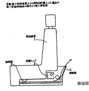
自動車の後部座席からの使用を前提とした場合の第一実施例構成の側方から視た断面図: The sectional view looked from the side of the 1st Example composition at the time of being premised on the use from the backseat of the car
